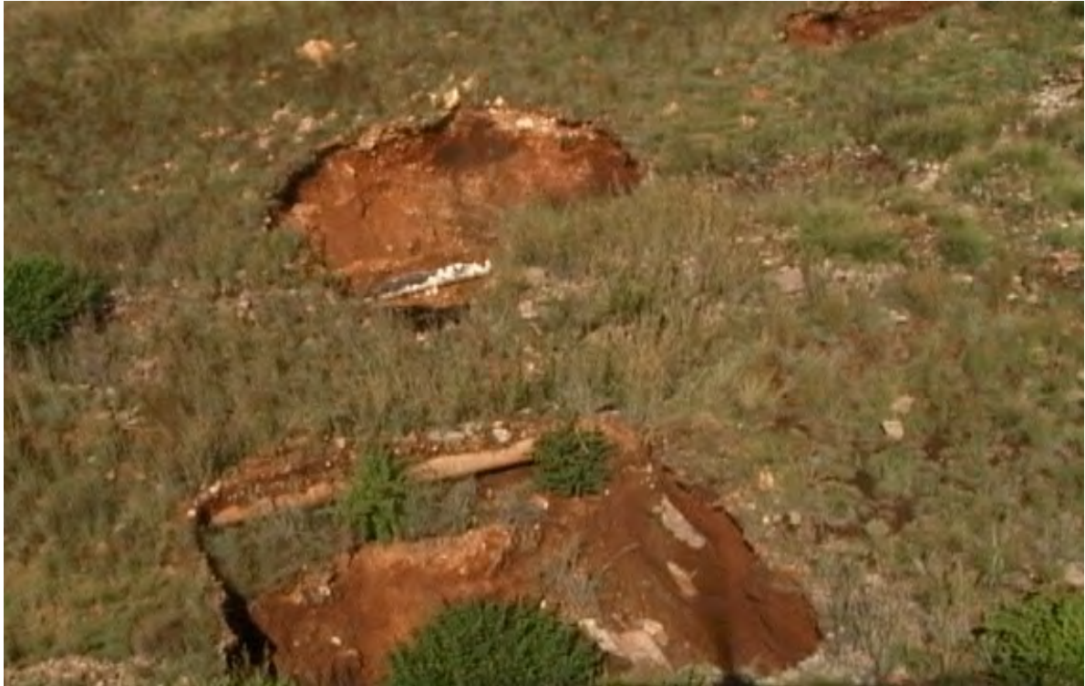
PLATE 5: SINKHOLE AS RESULT OF LEAKING WATER MAINS
