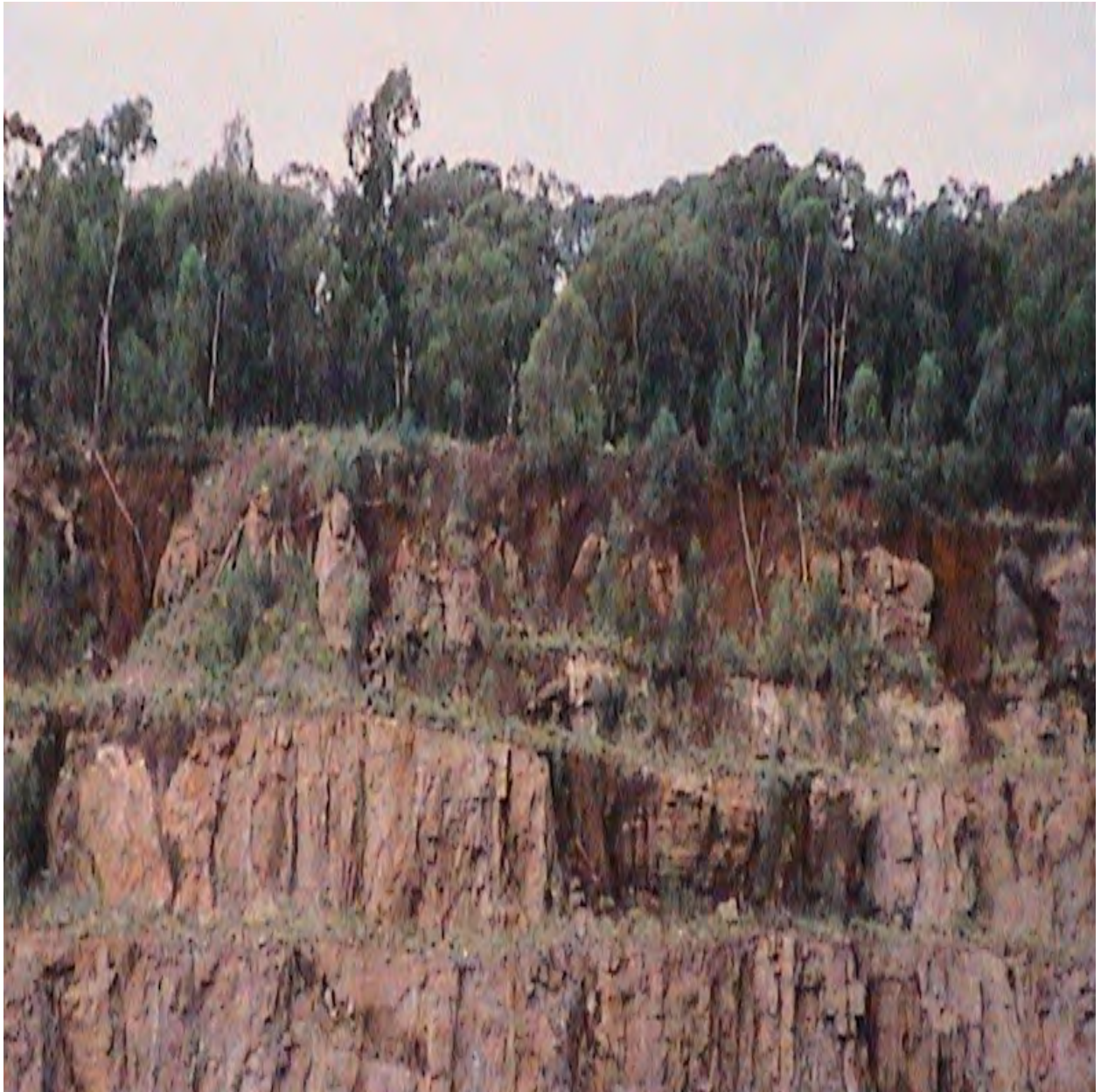
FIGURE 3: SUBSURFACE DOLOMITE PROFILE SHOWING PINNACLES AND SOIL FILLED FRACTURE ZONES
