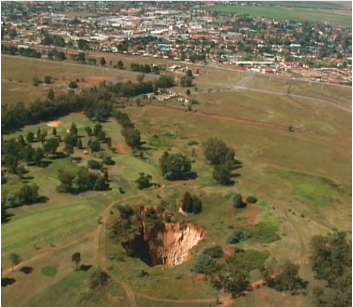
PLATE 7: LARGE SINKHOLE AS RESULT OF DEWATERING
