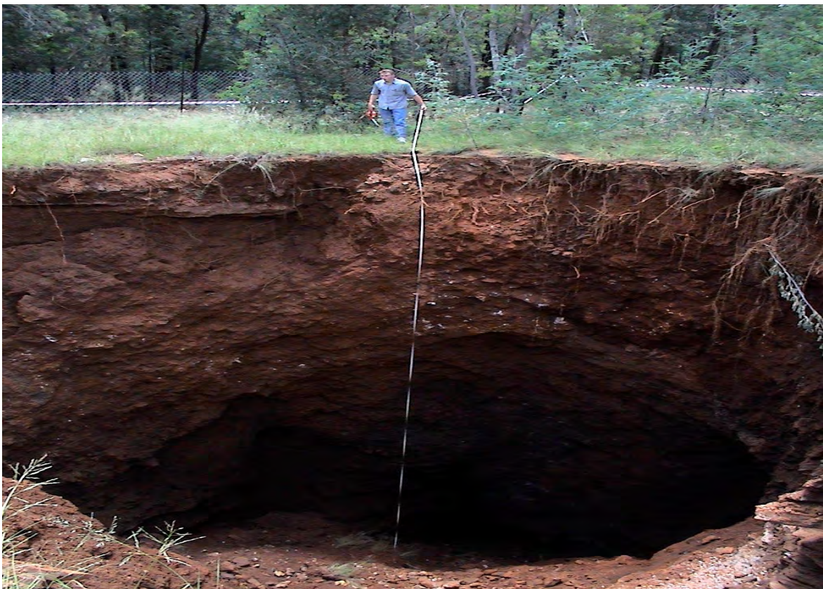
PLATE 4: SINKHOLE AS RESULT OF STORM WATER INGRESS
